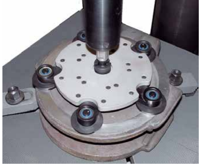
Grinding gate valve wedge with planet grinding disk
