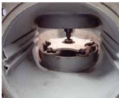
Grinding of gate valve
