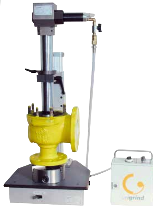
SVS 1 grinding a valve on machine stand
