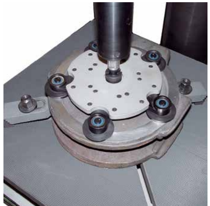
Grinding of gate valve wedge
