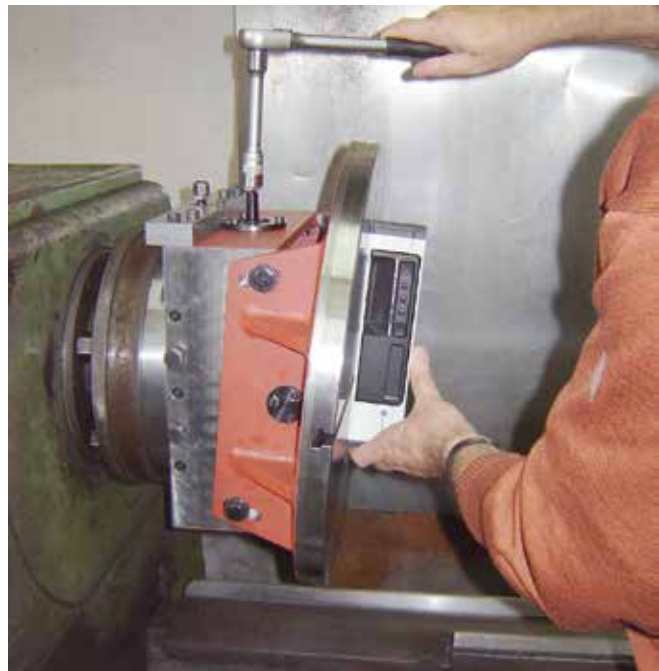
Adjusting the tilting angle with digital measuring device
