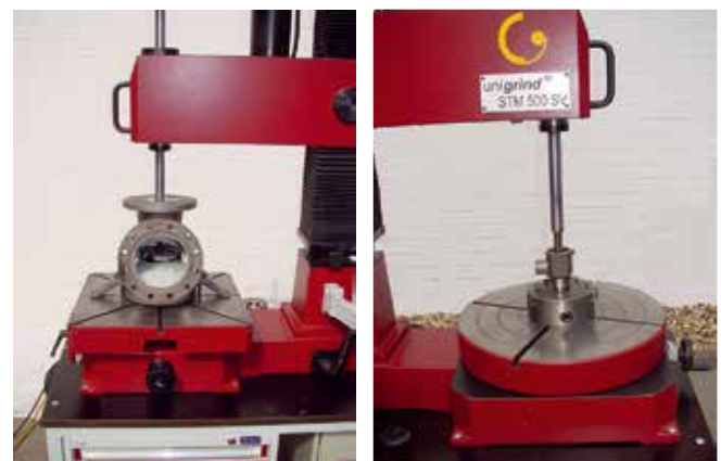
Grinding gate valve on tilting table
