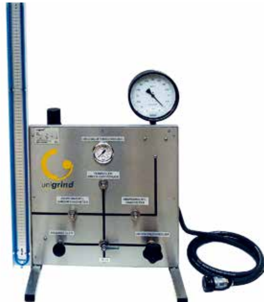
TSV portable vacuum test system and pressure test
